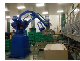
**new weighing and packaging** lines, as well as automisation of the process of palletising the melons and watermelons and tracking the fruit through the process.
